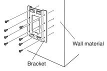
fig.1 Attaching the bracket
